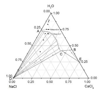
Figure 1. Confirm the Aspen plus solubility data with the phase diagram
