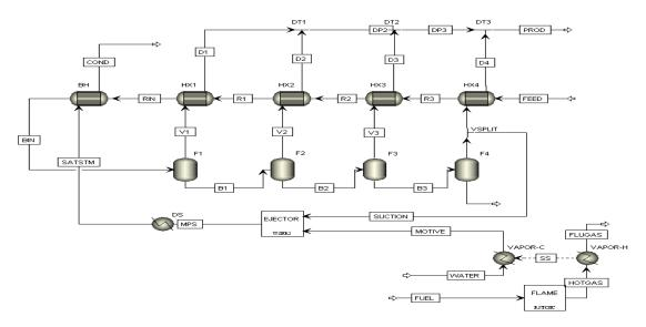
Figure 2. MSF desalination process
