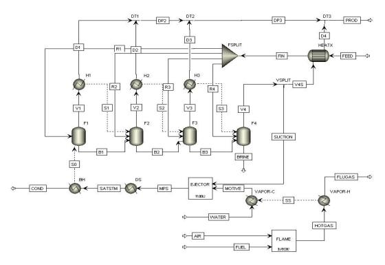
Figure 3. MED desalination process
